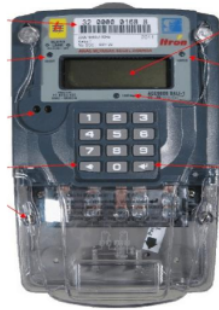
Gambar 2.19 Kwh Meter Digital
