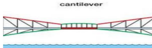
GAMBAR 2.5, Jembatan Cantilever Bridge/jembatan
