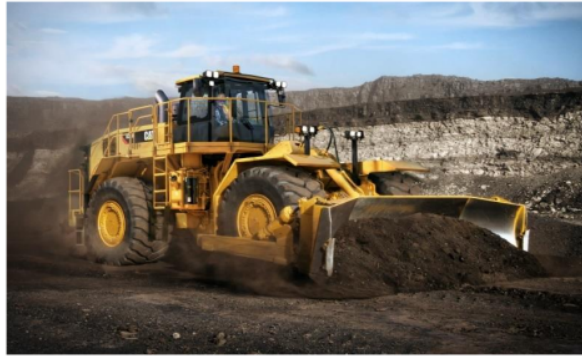
Gambar : wheel bulldozer
